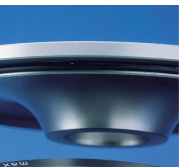
Angle rotors have a surrounding groove (1) above the tube boring which collects leaked liquids and aerosols which therefore cannot have an effect on the seal (2). The risk of spilling liquids is thus limited. This effect is supported by a liquid rejecter at the rotor lid (3) which, at the same time, holds the sealing ring.
