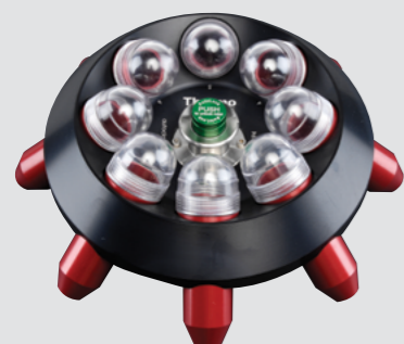
8 x 50 Individually Sealed Fixed Angle Rotor, 45°, R max 143 mm
