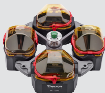
TX-1000 Swinging Bucket Rotor 1 , 90°, R max 209 mm
