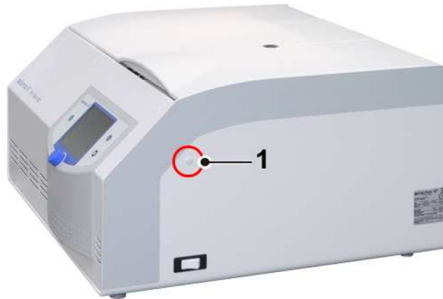
Fig. 28: Position of the opening for the emergency lid release
