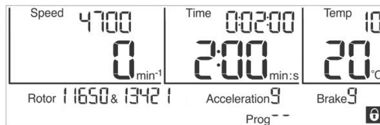
Fig. 25: "Padlock" symbol indicating an activated input lock
