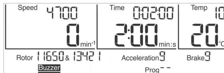
Fig. 21: The sound signal "Buzzer" is activated
