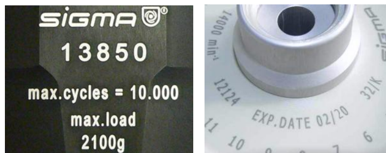
Fig. 4: Different service life – engraving on the bucket/rotor
