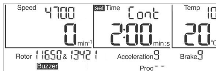
Fig. 14: Indication "Cont" during a continuous run
