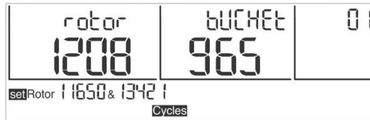
Fig. 23: Cycle display for rotor 11650 and bucket 13421
