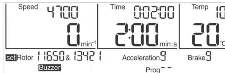
Fig. 18: Preselection of a rotor or a rotor/bucket combination
