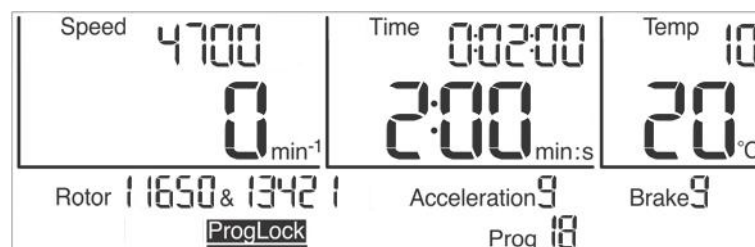
Fig. 22: The program lock "ProgLock" is activated
