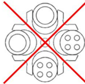
Fig. 7: Permissible and impermissible loading of a swing-out rotor with different tube sizes (example illustrations)
