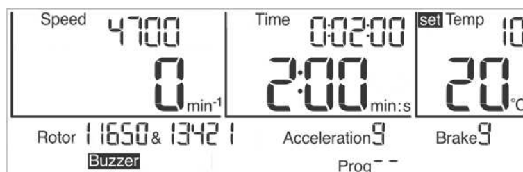
Fig. 15: Setting the temperature
