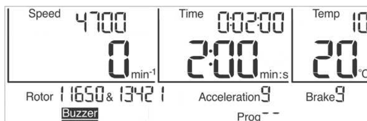
Fig. 20: The sound signal "Buzzer" is activated
