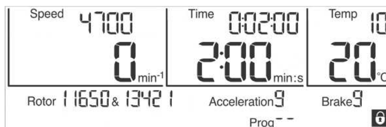
Fig. 24: "Padlock" symbol indicating an activated input lock
