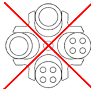
Fig. 6: Permissible and impermissible loading of a swing-out rotor with different tube sizes (example illustrations)
