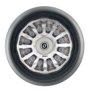
View into the centrifuging chamber showing the 1515-A rotor with 12 cyto inserts
