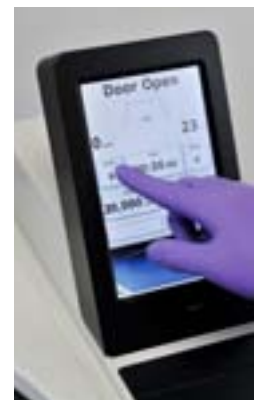
3. Confirm centrifuge program and begin run
