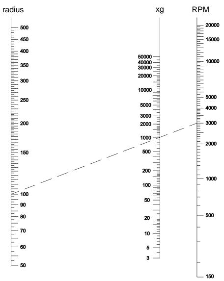
Total separating force applied to a sample in a centrifuge depends on the duration of the centrifuge run and on the RCF (relative centrifuge force) applied to the sample. RCF is generally calculated in units x gravity (x g). The diagram above allows you to graphically calculate RCF by drawing a line from the centrifugal radius (on left) to the speed (on right). The value of the RCF (xg) applied to the sample is approximated by the value at the point where the line crosses the "xg" axis (center).
