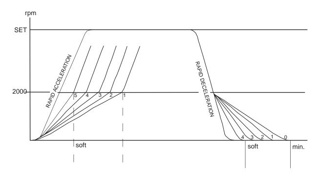
figure 5.4 Acceleration & Braking
