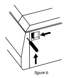
4. After the lid is open, replace the nylon screw.
