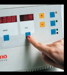
Set the required speed and the required time. With the "start" button, repeat runs can easily be recalled.
