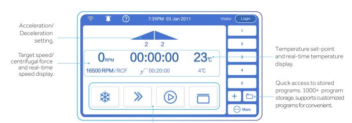
Clear one-touch buttons for fast refrigeration, fast centrifugation, intelligent start-stop and lid-closing status.
