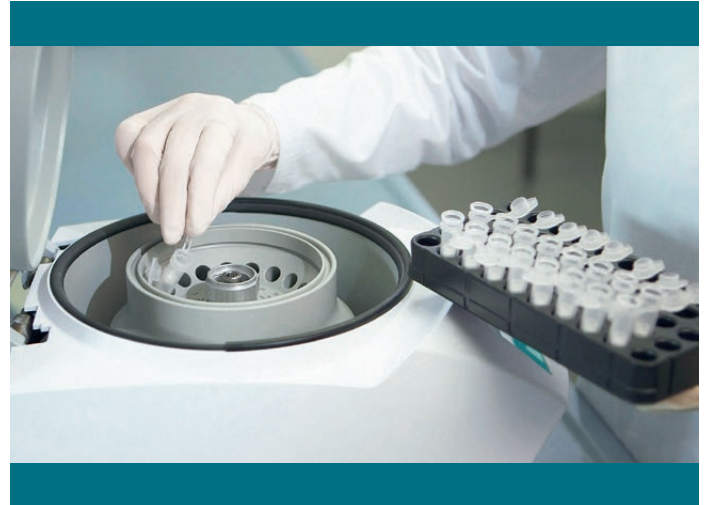
The MIKRO 185 (Cat. No. 1203) with spin column rotor (Cat. No. 1213) being used for sample preparation for PCR.
