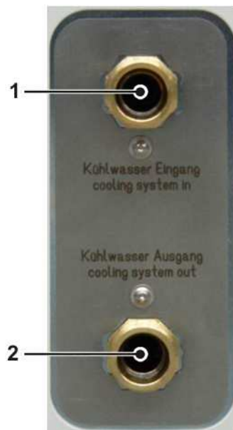
Fig. 17: Connections for the water cooling system
