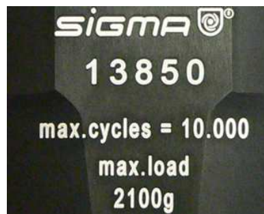
Fig. 8: Different service life – engraving on the bucket/rotor
