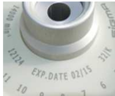
Fig. 8: Different service life – engraving on the bucket/rotor
