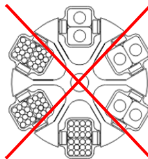
Fig. 18: Permissible and impermissible loading of a swing-out rotor with different tube sizes (example illustrations)
