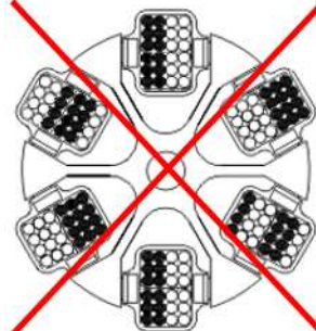
Fig. 8: Permissible and impermissible loading of an angle rotor and a swing-out rotor (example illustrations)
