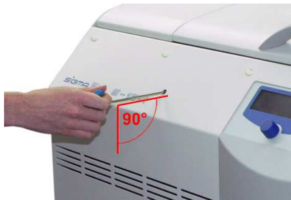
Fig. 30: The emergency lid release key must be inserted horizontally (similar to illustration)
