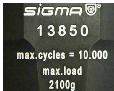
Fig. 4: Different service life – engraving on the bucket/rotor
