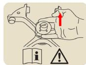
This Symbol refers to check, if the rotor is installed correct by lifting it slightly at the handle.
