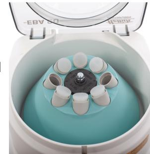
Step 3 — Ensure the pre-inserted fillers are not removed but pushed into the holes as far as possible and remain spaced as per picture right.
