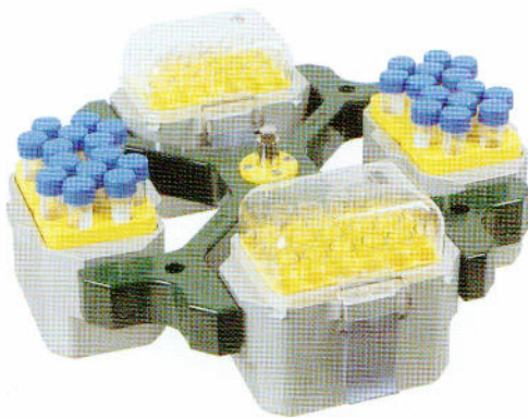
Swing-out rotor, \sphericalangle 90^\circ , 4-place, n = 4,500 \text{ min}^{-1} , RCF 4,754
