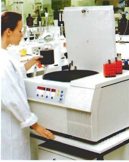
Megafuge 1.0 R – universal table-top centrifuge with refrigeration
