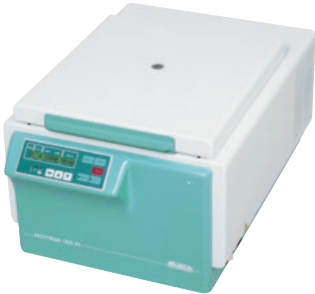
ROTINA 35 R benchtop centrifuge, refrigerated dimensions (H x W x D): 380 x 468 x 695 mm Cat.-No. 1710
