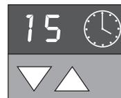
By pressing the key briefly, you increase or decrease the preset run time in steps of 0.1 min. This option is supposed to be used for small changes and fine tuning.
