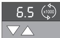
By pressing the key briefly, you increase or decrease the speed in steps of 100 rpm. This option is supposed to be used for small changes and fine tuning.
