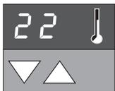
By pressing the key briefly, you increase or decrease the temperature in steps of 1 °C. This option is supposed to be used for small changes and fine tuning.
