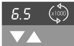
By pressing the selected key **briefly**, you increase or decrease the speed in steps of 100 rpm. This option is supposed to be used for small changes and fine tuning.
