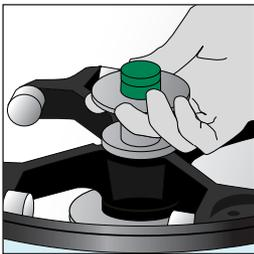
Push center button to remove rotor
