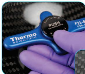
Auto-Lock is identified on Thermo Scientific superspeed centrifuges with a **black push button** and on Thermo Scientific general purpose centrifuges with a **green push button**.
